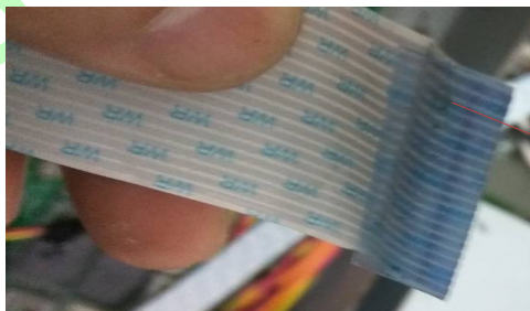
Pelindung kabel FFC (plastic berwarna biru)
